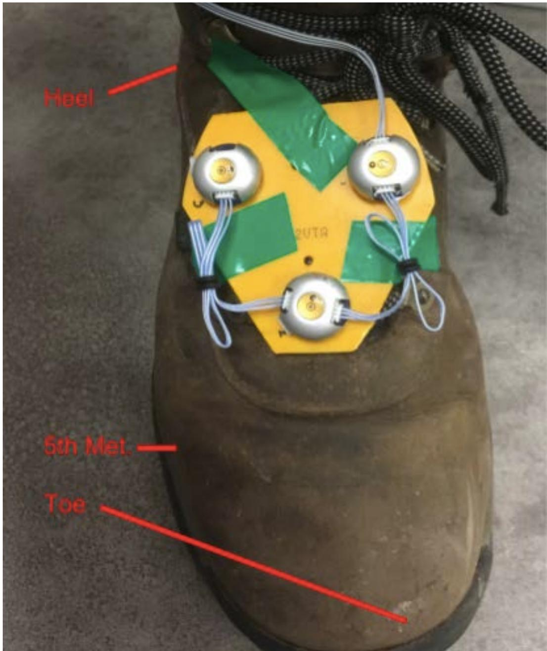
Figure 9. Placement of the rigid body on the upper foot, and the locations of the digitized landmarks of the heel, big toe, and 5th metatarsal.
