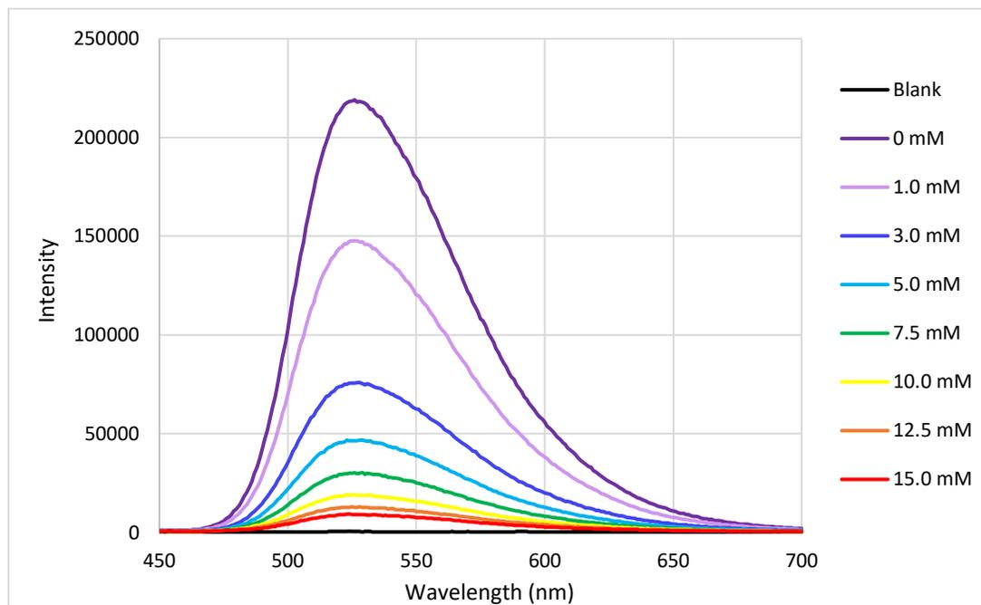
**Figure 5.9:** Fluorescence titration of vitamin B2 with SCX4 at 55°C.
