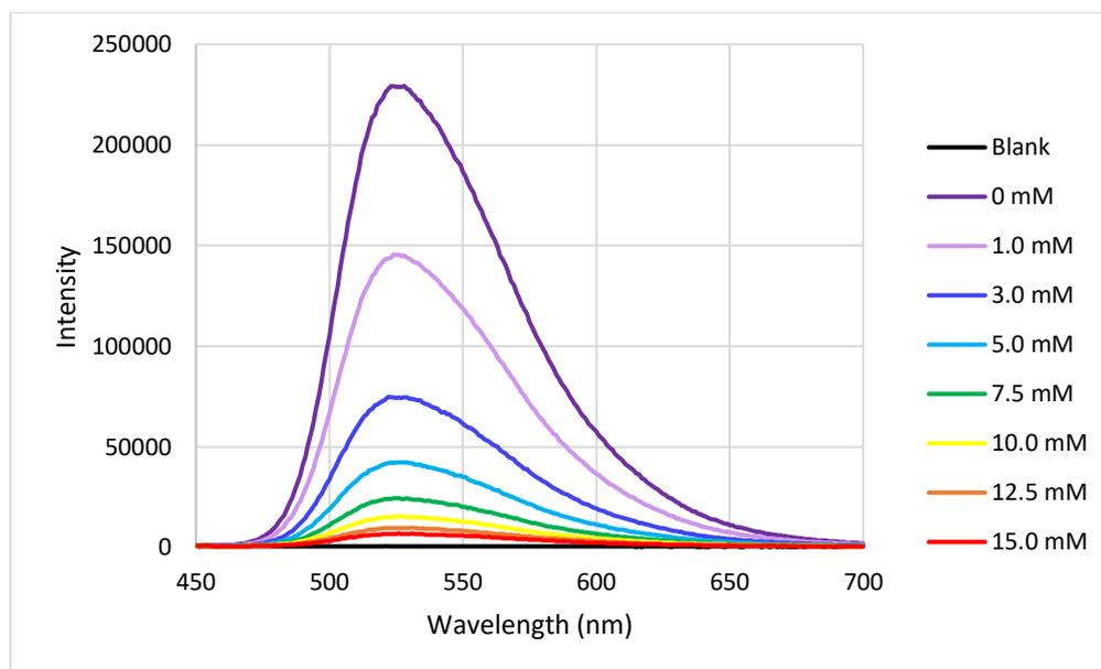
**Figure 5.5:** Fluorescence titration of vitamin B2 with SCX4 at 35°C.
