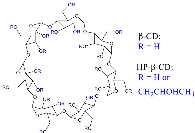
**Figure 1.3:** Chemical structure of  $\beta$ -CD and HP- $\beta$ -CD.
