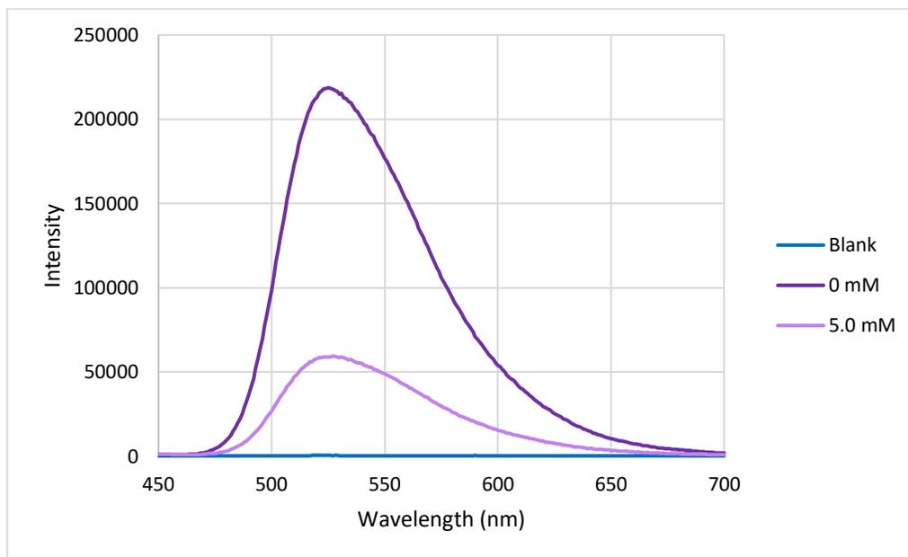
**Figure 3.3:** Emission spectrum of vitamin B2 with and without 5.0 mM SCX6.
