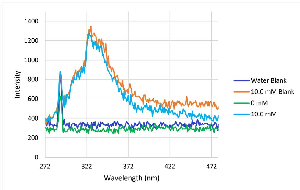
**Figure 3.1:** Emission spectrum of vitamin B3 with and without 10.0 mM HP- $\beta$ -CD.
