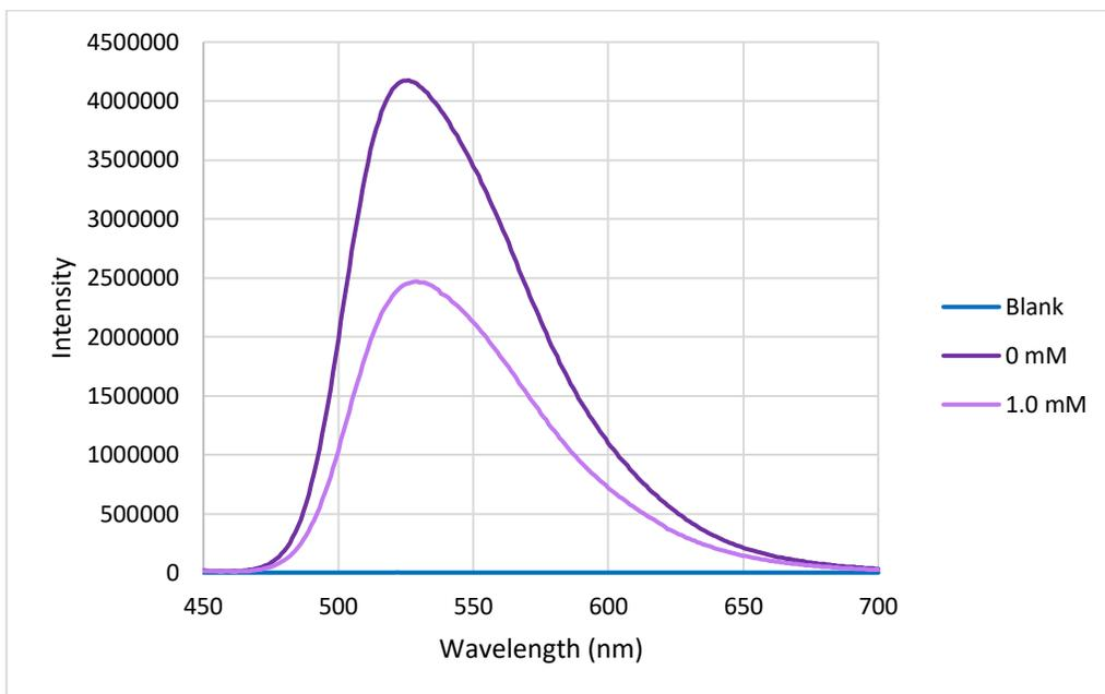
**Figure 3.5:** Emission spectrum of vitamin B2 with and without 1.0 mM CB7.
