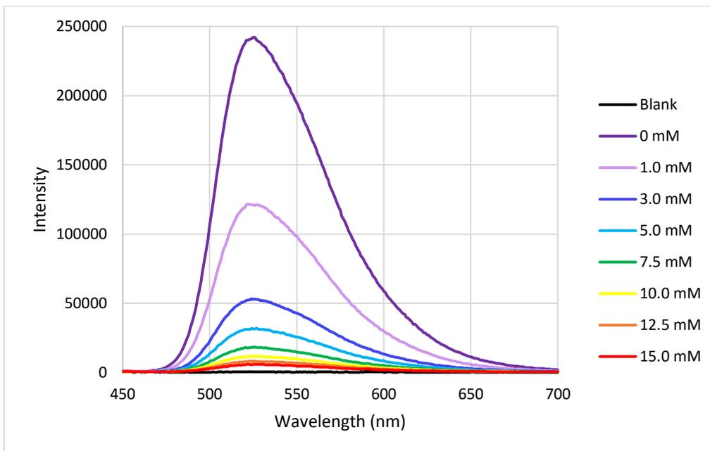
**Figure 5.1:** Fluorescence titration of vitamin B2 with SCX4 at 7°C.
