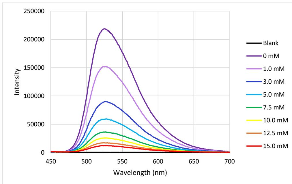
**Figure 4.1:** Fluorescence titration of vitamin B2 with SCX6.
