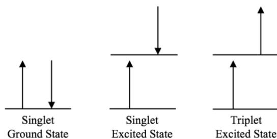
**Figure 1.6:** Schematic diagram of singlet and triplet state electronic excitations.
