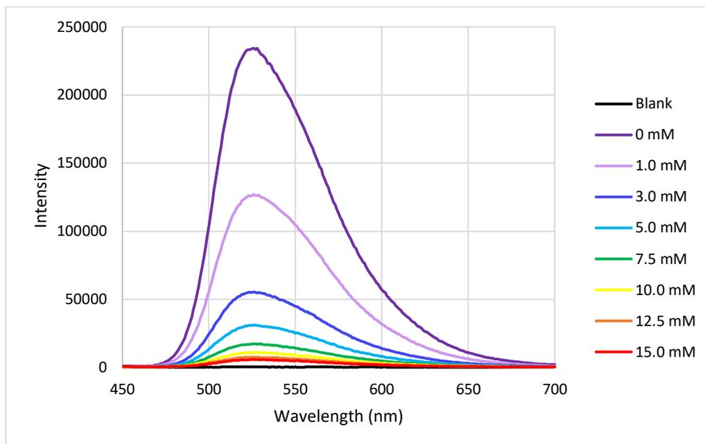
**Figure 5.3:** Fluorescence titration of vitamin B2 with SCX4 at 15°C.
