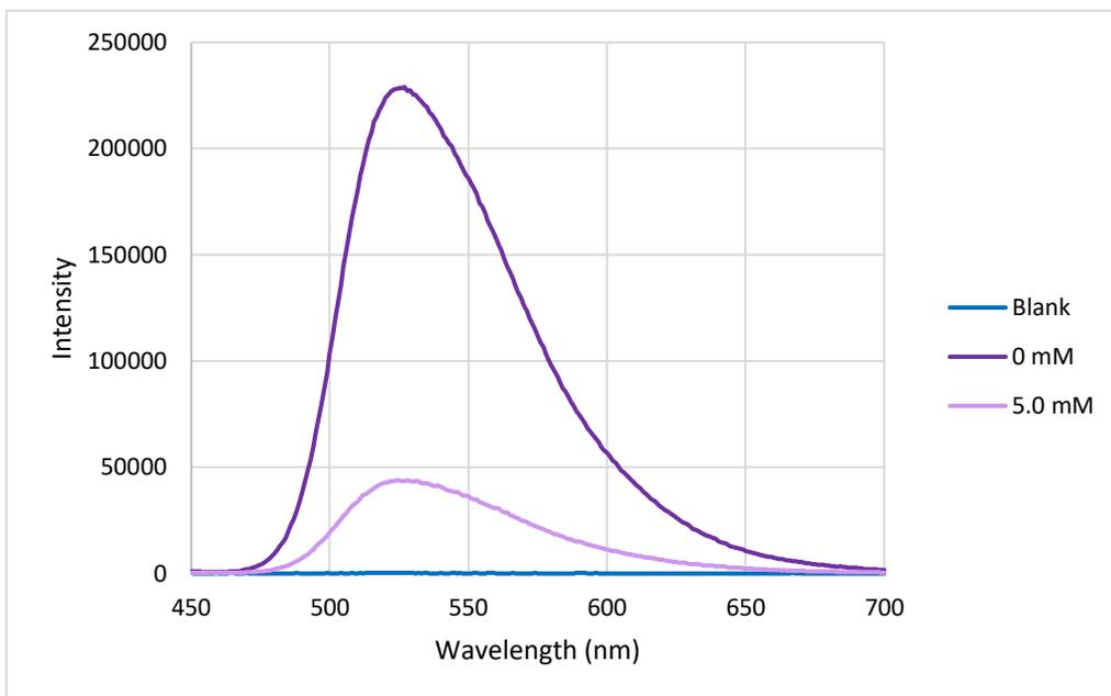
**Figure 3.4:** Emission spectrum of vitamin B2 with and without 5.0 mM SCX4.
