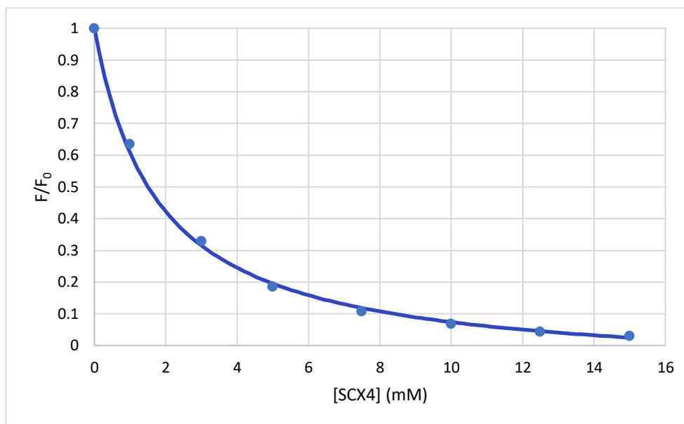
**Figure 5.6:**  $F/F_0$  versus the concentration of SCX4 with vitamin B2 at 35°C.
