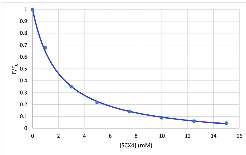
**Figure 5.10:**  $F/F_0$  versus concentration of SCX4 at 55°C.
