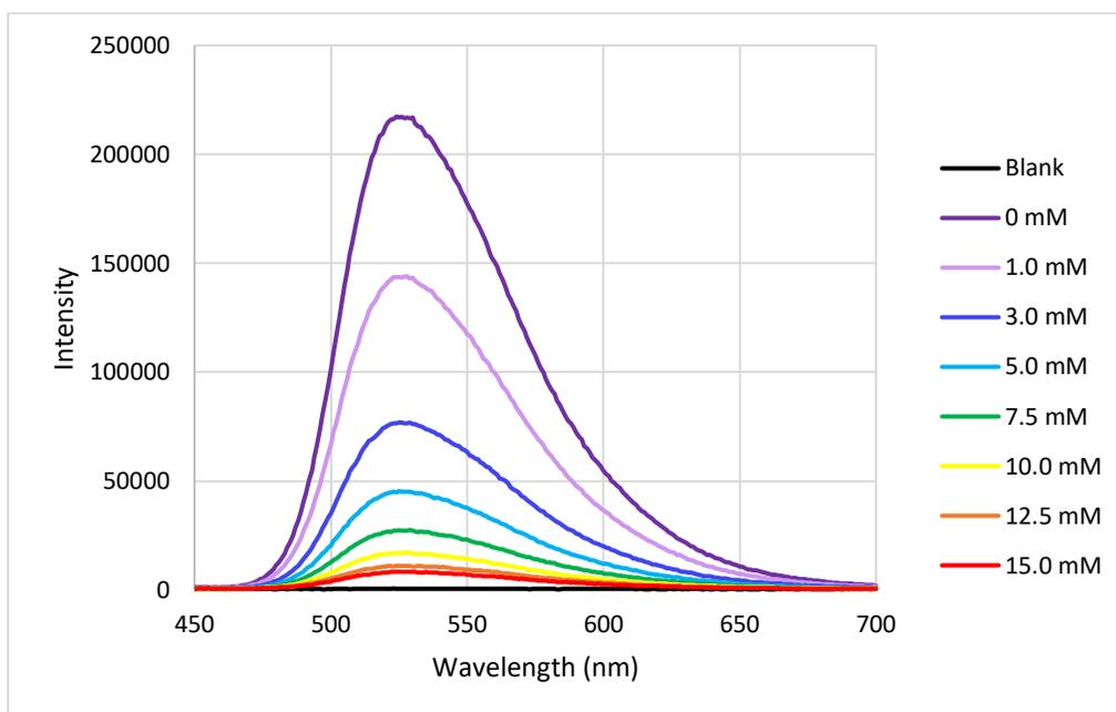
**Figure 5.7:** Fluorescence titration of vitamin B2 with SCX4 at 45°C.
