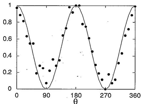
FIG. 7. TPF signal for TMA as a function of  $\theta$  for  $t_d=0$ . ●, experimental; —,  $\cos^2 \theta$  normalized to highest experimental value.
