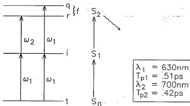
FIG. 2. Model for the TPF for TMA. The relevant states  $S_0$ ,  $S_1$ , and  $S_2$  are represented by one (1), one ( $i$ ), and two levels ( $q, r$ ), respectively. The relevant experimental laser wavelengths and pulse widths are also indicated on the figure.
