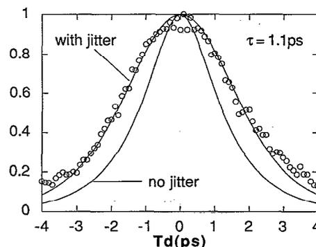
FIG. 4. TPF signal for azulene as a function of  $t_d$  for  $\hat{e}_1 = \hat{e}_2$ .  $\circ$ , experimental; —, theory with  $\tau = 1.1$  ps both with and without jitter.
