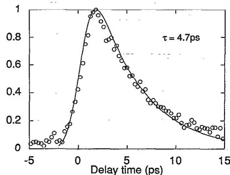
FIG. 5. TPF signal for TMA as a function of  $t_d$  for  $\hat{e}_1 = \hat{e}_2$ .  $\circ$ , experimental; —, theory with  $\tau = 4.7$  ps including jitter.
