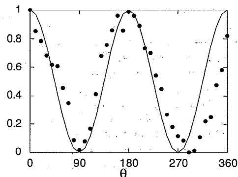
FIG. 6. TPF signal for azulene as a function of  $\theta$  for  $t_d=0$ . ●, experimental; —,  $\cos^2 \theta$  normalized to highest experimental value (see main text).
