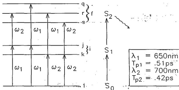
FIG. 1. Model for the TPF for azulene. The relevant states  $S_0$ ,  $S_1$ , and  $S_2$  are represented by one (1), two ( $j, k$ ), and the three levels ( $q, r, s$ ), respectively, under the assumptions discussed in the main text. The relevant experimental laser wavelengths and pulse widths are also indicated on the figure.
